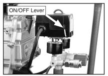
Figure 4. ON/OFF lever.
